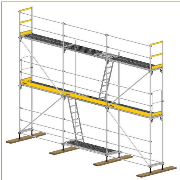
Figure 39: Completing the Upper Guardrails
