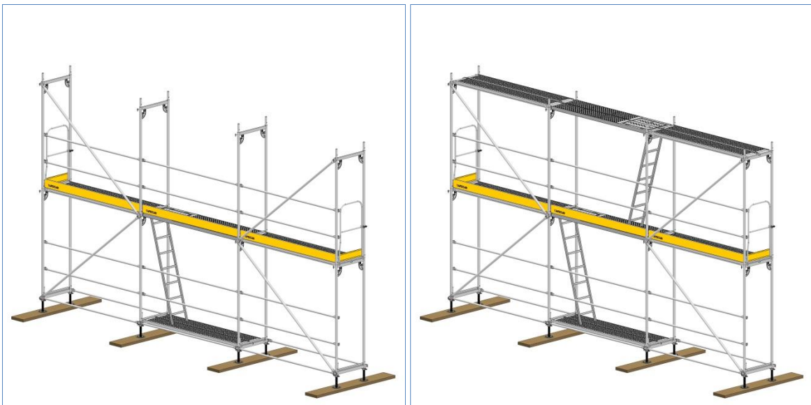
Figure 34:Completing Side Guardrails and Toes Figure 35:Fitting Last Deck Platforms
