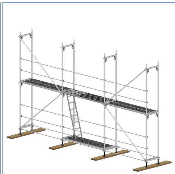
Figure 27: Completing Upper Rods
