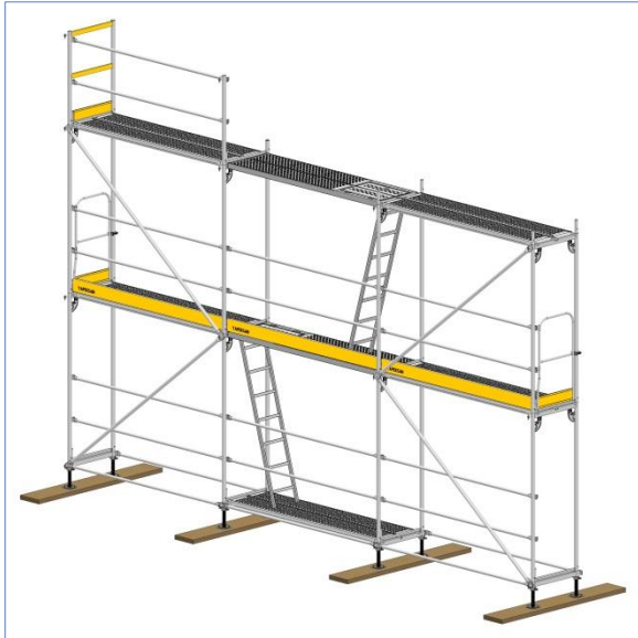
Figure 37: Fitting the Upper Guardrail Horizontal Connections
