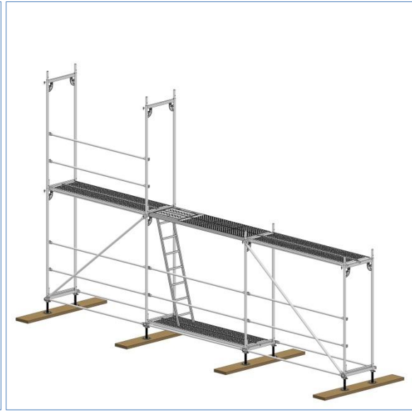
Figure 25: Fitting Upper Deck Horizontal Connections
