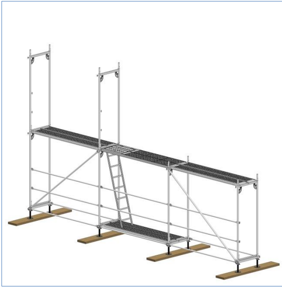
Figure 24: Fitting Upper Deck Frames
