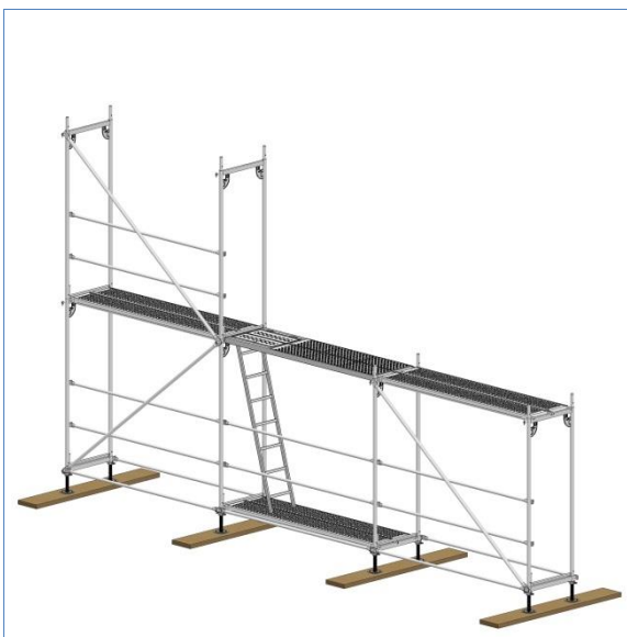
Figure 26: Fitting Upper Diagonal Connections
