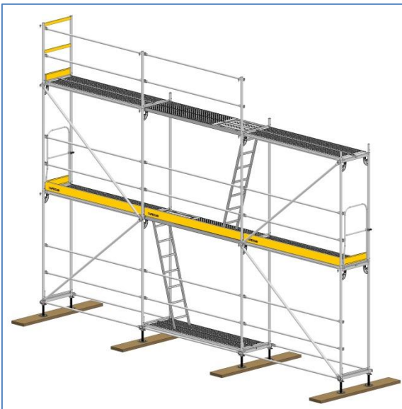
Figure 38: Completing the Upper Guardrail Horizontal Connections
